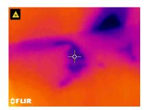
**Fig. 5-7(a)** Laser and Crosshairs visible; Aim the Laser at the test surface
